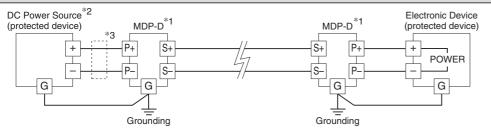
The MDP-D is not applicable to protect two-wire transmitters. To protect two-wire transmitters model MDP-24-1 designed to yield only small leakage current is suitable.
