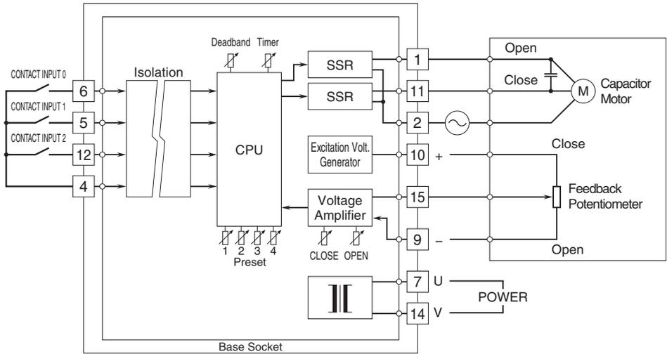
Note: Note that when limit switches inserted in motor wiring, the making/breaking may cause stress on the SSRs.
