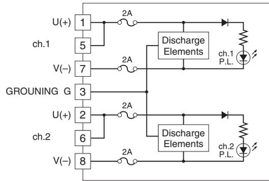
Make sure to connect a DC power source in the proper polarity in order to turn the LED on.
