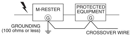
A crossover wire between M-RESTER ground and ground or metallic housing of equipment is required for protection.
