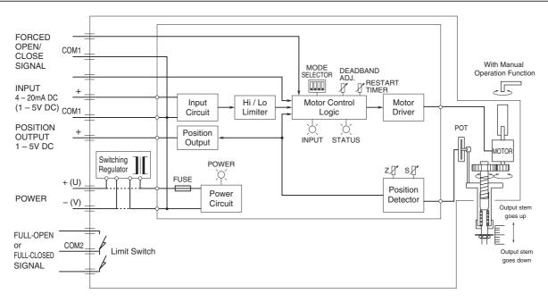
Full-open/-closed signals and forced open/close signals are optional. Disregard the switching regulator circuit for DC power input.
