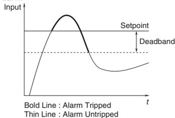
■ **LOW ALARM:** When the signal input goes below the preset setpoint, the relay provides a tripped condition.
