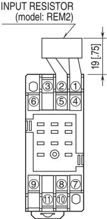
Input shunt resistor attached for current input.
