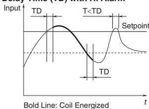
■ **POWER ON DELAY TIME:** The relay does not provide a tripped condition for a duration of the preset Power ON Delay Time (TDP) after the power supply is turned on, even when the signal input is in an alarm range.
