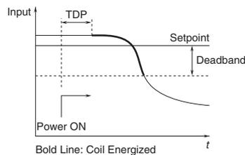
■ **LATCHING OUTPUT:** The relay does not return to an untripped condition once the signal input goes across the threshold, unless:
