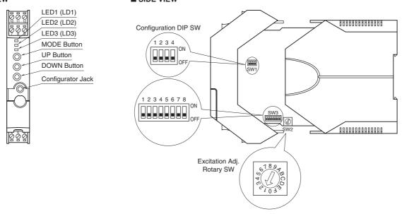
The DIP switch setting is required to select output types before setting a precise output range using the PC configurator software.
