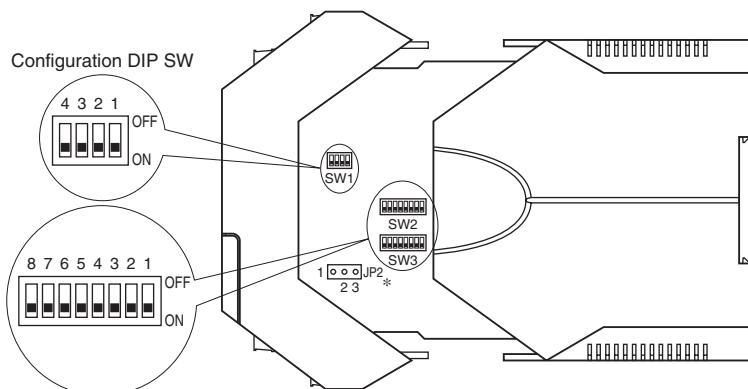
\*For Voltage Input (V) range, switch the JP2 jumper to the 2 – 3 position.
