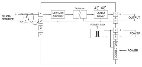
This unit, by its fast-response feature, is not designed to eliminate noise present in the input signal. Use a shielded twisted-pair cable to prevent noise from entering through the input wiring.
