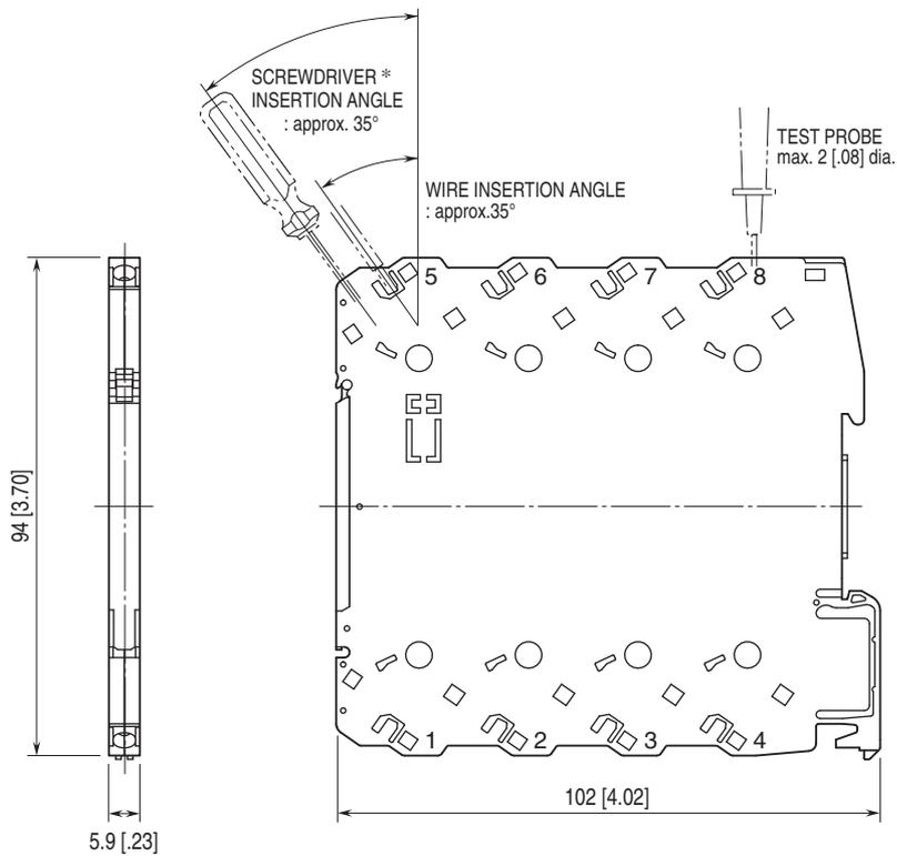
\*Use a minus screwdriver: tip width 3.8 mm max., tip thickness 0.5 to 0.6 mm
