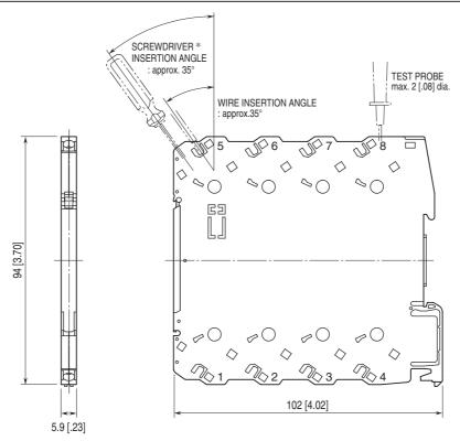
$^*\mbox{Use}$  a minus screwdriver: tip width 3.8 mm max., tip thickness 0.5 to 0.6 mm
