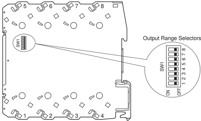
The output signal type is configurable with the DIP switches. Refer to the installation manual for detailed procedure.
