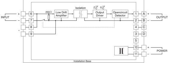
\*Use the terminals 6 - 7 for input. The terminals 8 - 9 can be used but the opencircuit detection is canceled.
