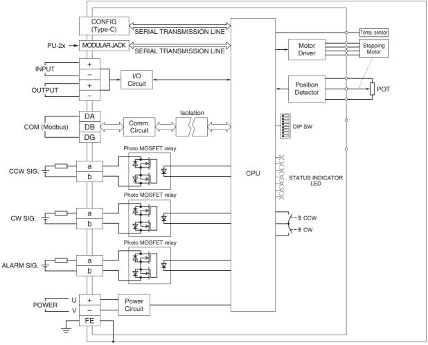
Note1: No polarity between a and b.
