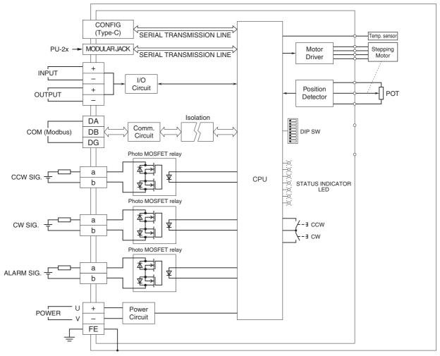
Note1: No polarity between a and b.
