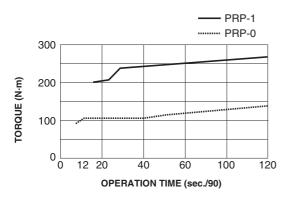
Note: Operational torque for PRP-0 is 100 N·m. Operational torque for PRP-1 is 200 N·m.
