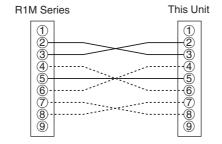
The above connection including solid and broken lines is an example of 'Interlink' cable.
