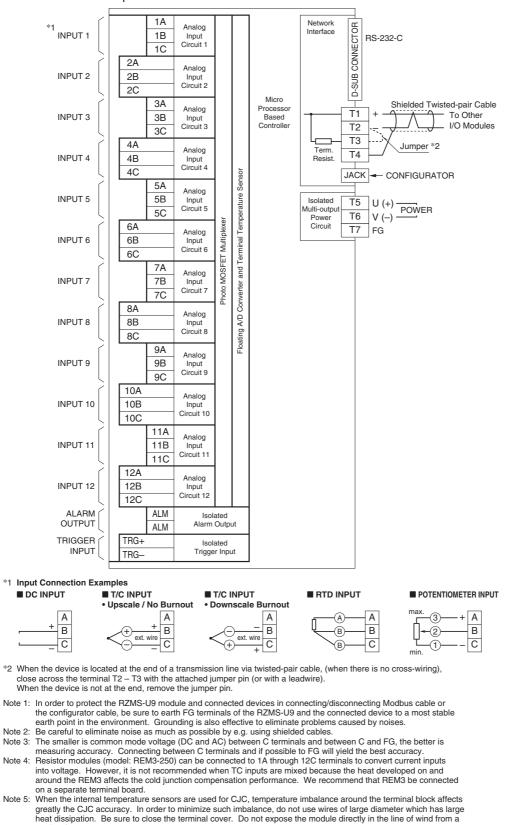
Two-wire RTD can be used by closing across B and C terminals. Be sure to compensate wire resistance by
