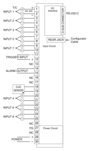
Note 1: DO NOT connect the terminals 13, 16, 17, 26 and 28 (NC: No Connection).
