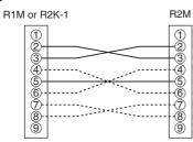
The above example with solid and broken lines shows an 'interlink' type cable.
