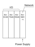
Single network module with external power supply module
