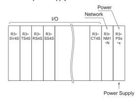
Single network module with two external power supply modules
