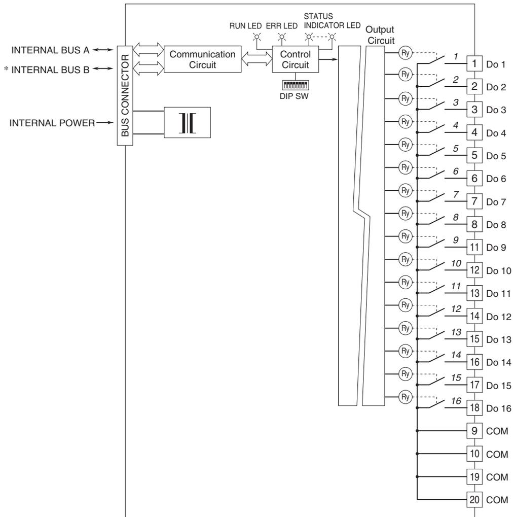
Numbers in italic indicate LED No.s assigned to the front panel LEDs.
