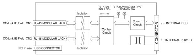
CN1 and CN2 of RJ-45 modular jacks for CC-Link IE Field network can be connected in any order.
