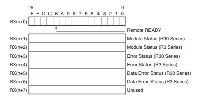
• RX(n+0)0 to 7 is reservation area, RX(n+0)B is used as Ready signal, the bit is "1" when this module is in normal.
