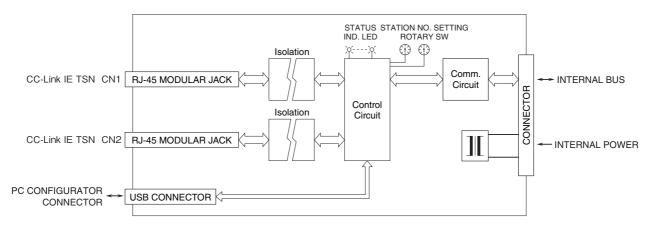
Regarding CN1 and CN2 of RJ-45 connector for CC-Link IE TSN network, there is no restriction for connection order.
