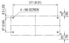
\*Working space required for mounting/unmounting the modules.
