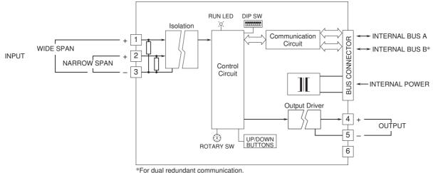
Note: Connect either wide or narrow span terminals for each channel.
