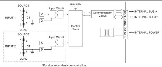
Note: The section enclosed by broken line is with 2-ch. option.
