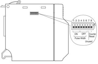
Counter Reset SW is normally OFF during operation.
