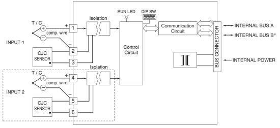
\*For dual redundant communication. Note: The section enclosed by broken line is with 2-ch. option.
