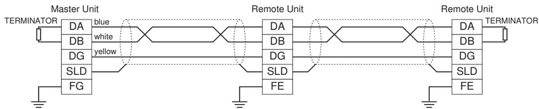
Be sure to connect the terminating resistor across DA and DB at both ends of communication line.
