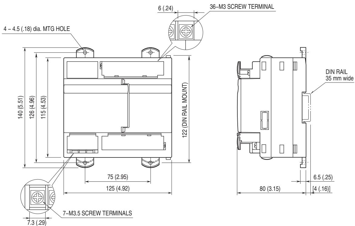
**MOUNTING REQUIREMENTS unit: mm [inch]****■ SINGLE MOUNTING**
