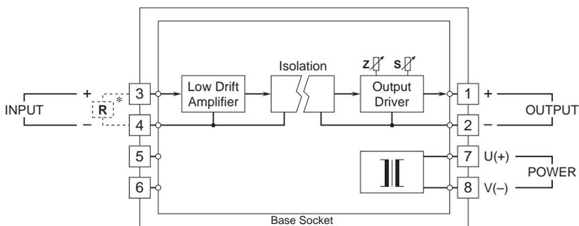
\*Input shunt resistor attached for current input.
