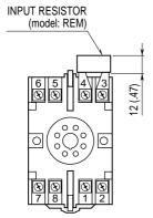
Input shunt resistor attached for current input.
