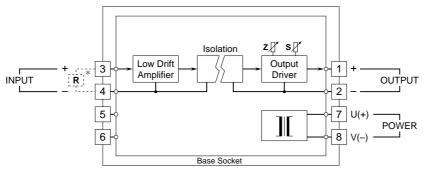
\*Input shunt resistor attached for current input.
