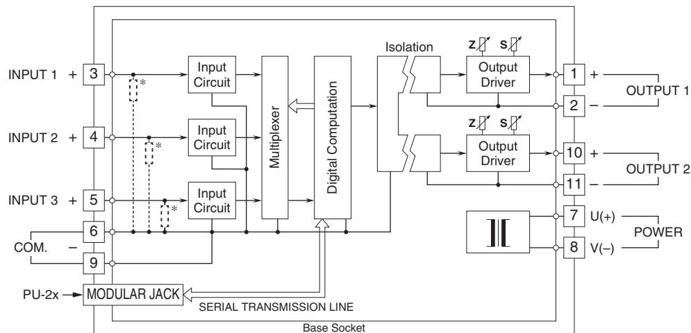
\*Input shunt resistor incorporated for current inputs.
