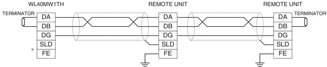
\* Connect SLD and FE for reducing noise interference if necessary.
