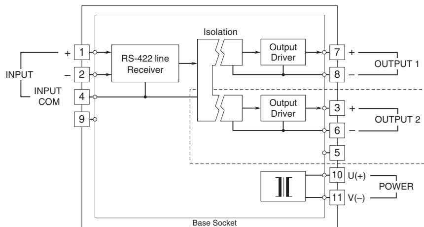
Note: The section enclosed by broken line is only with 2nd output option.
