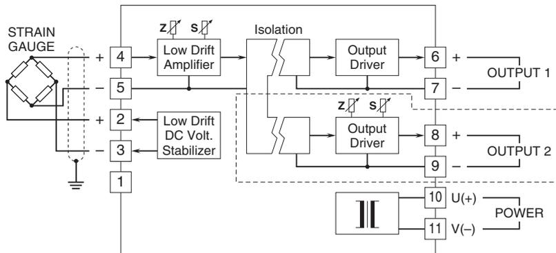
Note 1: The section enclosed by broken line is only with 2nd output option.
