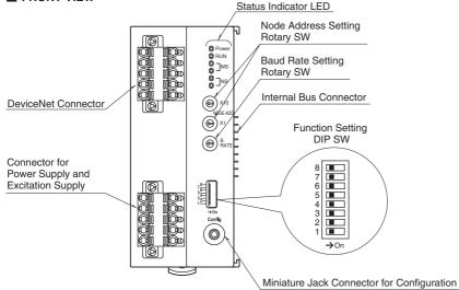
STATE COLOR TO INDICATE Green ON Power supplied ON / Blink Turns on or blinks depending on the status Green ON Green Normal operation ON Red Critical failure Blink Minor failure Green Connections are established ON
