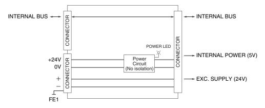
Internal bus is connected for the modules near to the power/network module out of the modules connected to the R8-PS1. Internal power and Exc. supply are not connected. All modules far from the power/network module are connected.
