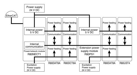
Note1. Use same power supply for the power/network module and extension power supply module. Note2. Max. 2 extension power supply module can be used at the same time.
