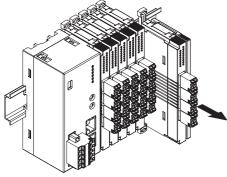
• Removing an intermediate module
