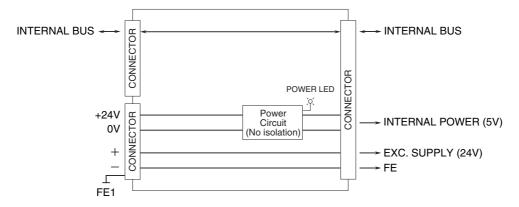
Internal bus is connected for the modules near to the power/network module out of the modules connected to the R80PS1. Internal power and Exc. supply are not connected. All modules far from the power/network module are connected.
