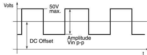
**Two-wire current pulse waveform**
