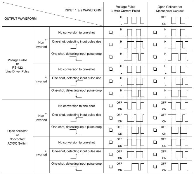
The pulse width in one-shot means the bold lined section of a pulse waveform. \*1. Specified by model number suffix code.
